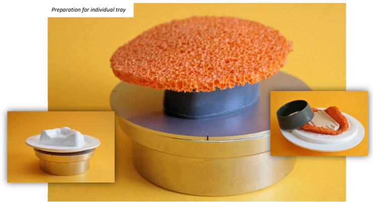
Adjust the silicone ring around the model so that the thicker part is in contact with the metal disc. This is to facilitate extraction once the thermoforming and cooling cycle has finished
