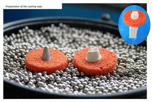
To print the casting caps use dedicated sponges (about 1 cm in diameter). Insert the abutment in the center of the sponge until the preparation edge emerges and place them in the basket. Use the pre-shaped sponges to avoid contact between the disc and the balls during thermoforming.
