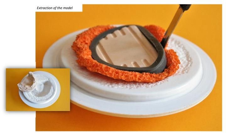
After thermoforming, with the aid of an instrument, remove the silicone gasket: the space left by the silicone ring will be used to facilitate the subsequent extraction of the plaster model.
